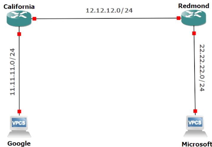
We just need to setup the interfaces with proper IP addresses, and then write the ip routes. Here is a more detailed image of the project with interface identifiers and chosen example IP addresses for each interface.
